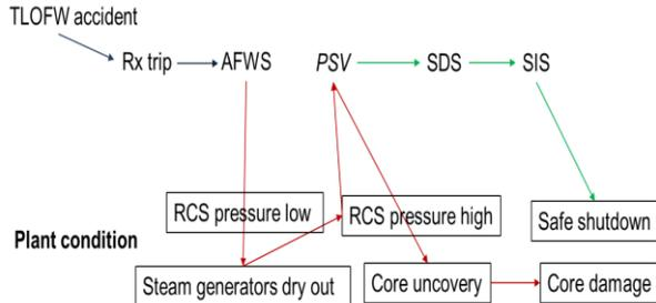
Fig. 1 Relationship between accidents, mitigation functions and plant condition in the case of TLOFW accident
