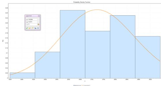
Fig. 5 Distribution of available time for diagnosis to initiate F&B operation under TLOFW accident without LOCA.
