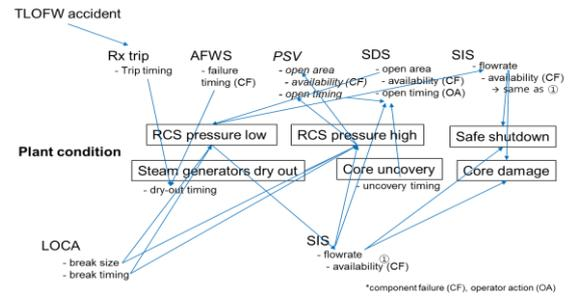
Fig. 3 Relationship between plant component, operator action, and plant condition in the case of TLOFW accident with LOCA
