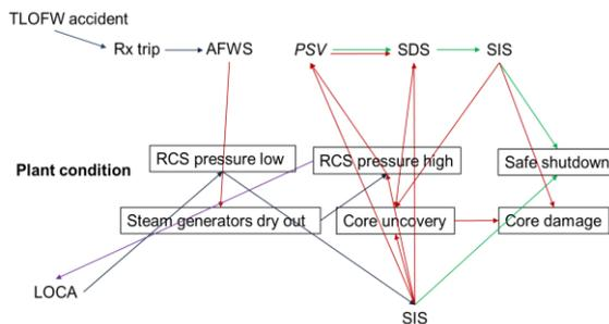
Fig. 2 Relationship between accidents, mitigation functions and plant condition in the case of TLOFW accident with LOCA
