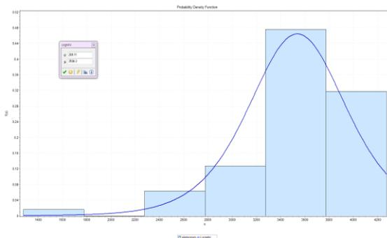
Fig. 4 Distribution of available time for diagnosis to initiate F&B operation when one HPSI pump is available under TLOFW accident with LOCA.
