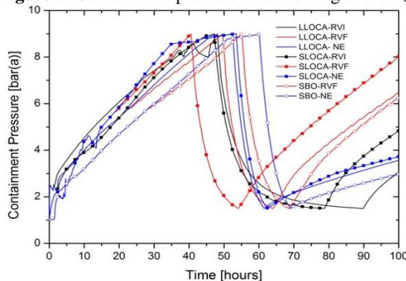
Figure 3. Containment pressure with Venting at 9 bar(a)
