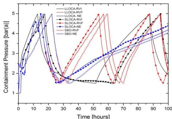
Figure 1. Containment pressure with Venting at 5 bar(a)
