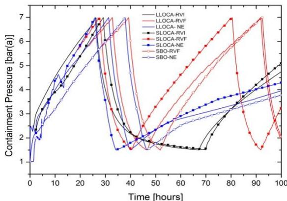
Figure 2. Containment pressure with Venting at 7 bar(a)
