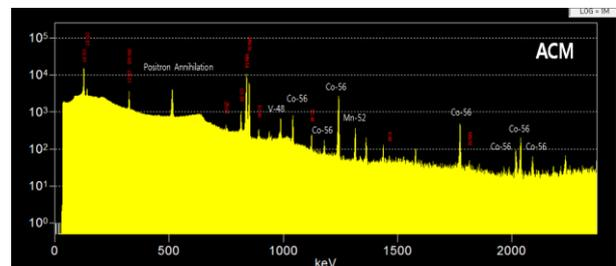
Figure 2. X-ray spectrum of AC magnet(ACM)
