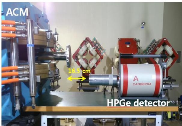
Fig. 1. Set of HPGe detector and AC magnet(ACM) of 100 MeV beamline
