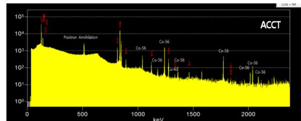
Figure 3. X-ray spectrum of ACCT
