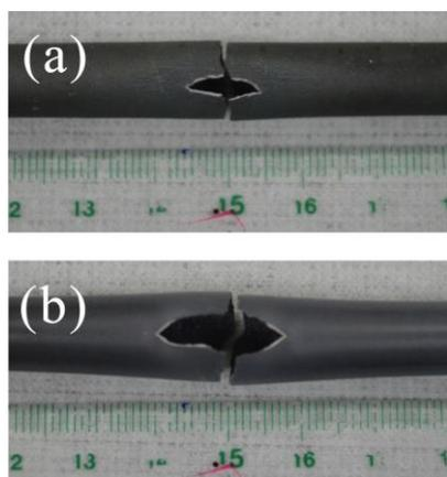
Fig. 2. Frontal view of burst opening of (a) Cr coated ATF and (b) existing Zr alloy tube samples after integral LOCA test.
