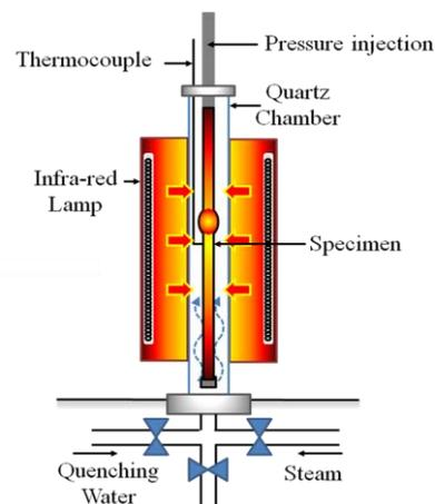
Fig. 1. Schematic illustration of the integral LOCA test facility.
