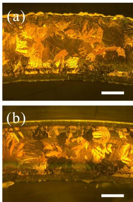
Fig. 3. Cross sectional micrographs 180° from the burst opening of (a) the Cr coated ATF and (b) Zr alloy tube samples after integral LOCA test. The bars indicate 200  $\mu\text{m}$  in length.
