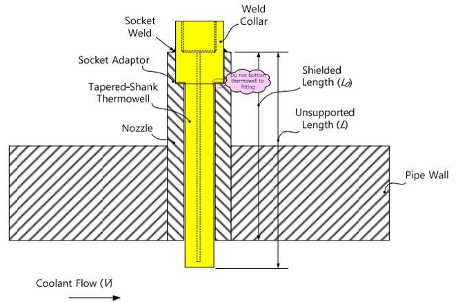
Fig. 4 Installation configuration of new thermowells in the facility
