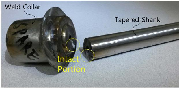
Fig. 3 Cracked thermowell (Weld collar and tapered-shank)
