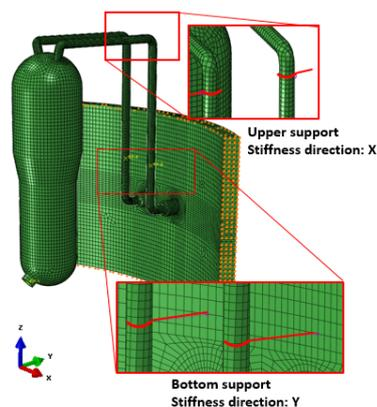
Fig. 1 Combined FE model and location of piping supports
