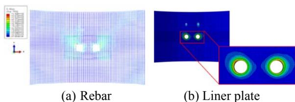
Fig. 2 von Mises stress contours when both supports fail
