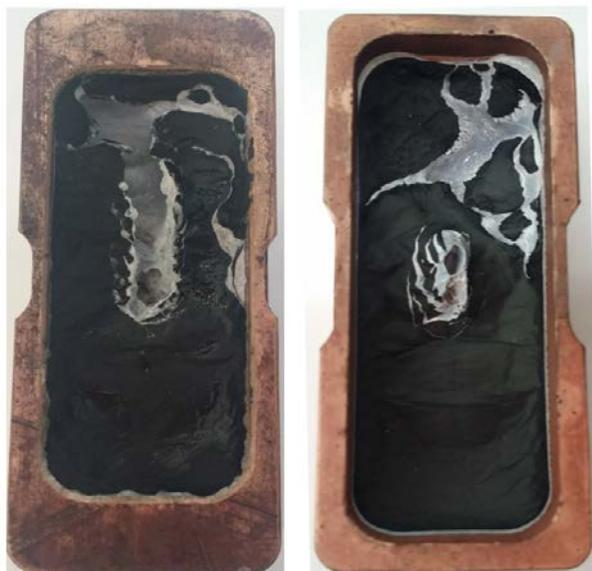
Fig. 5. Sodium surfaces after reaction test at 500 °C; (a) 10 cm<sup>2</sup>, (b) 12 cm<sup>2</sup>
