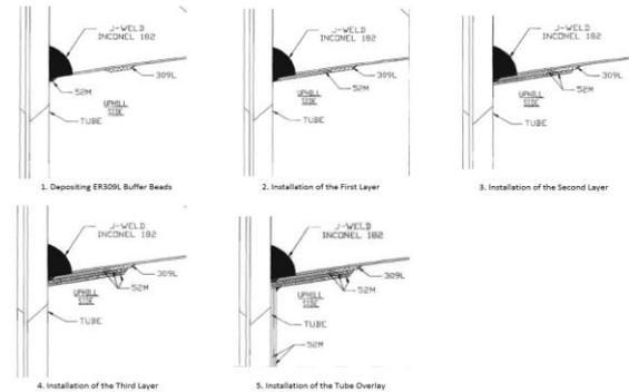
Figure 1 Welding Process of EFR
