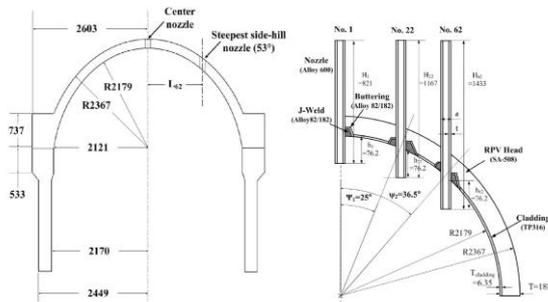
Figure 3 RPV upper head geometry details (mm)
