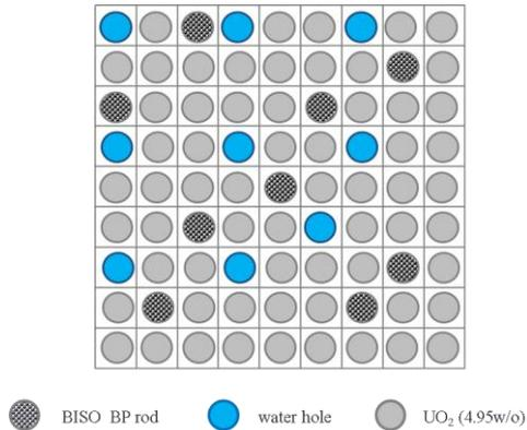
Fig. 1. Configuration of the new fuel assembly (1/4)
