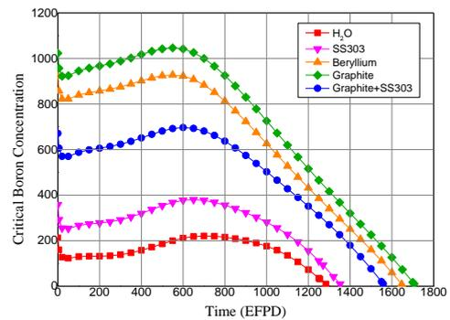
Fig. 4. Comparison of the evolutions of CBC over time for different radial reflectors
