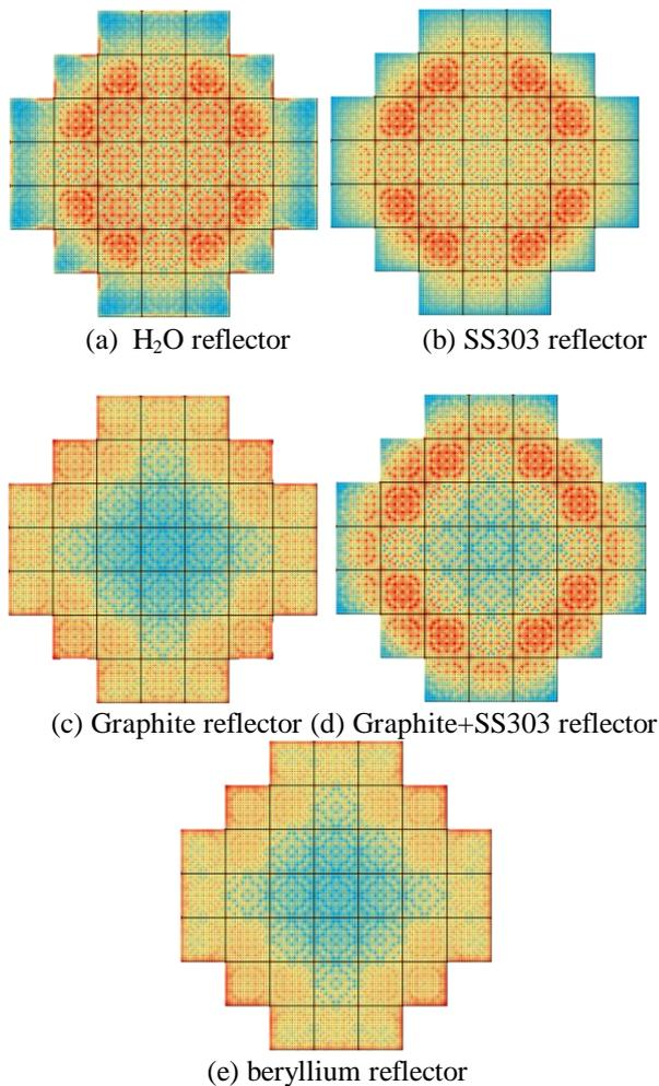
Fig. 5. Comparison of the fuel pin-wise thermal fluxes
