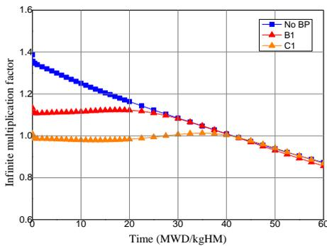
Fig. 2. Comparison of the evolutions of k-infs for new fuel assemblies
