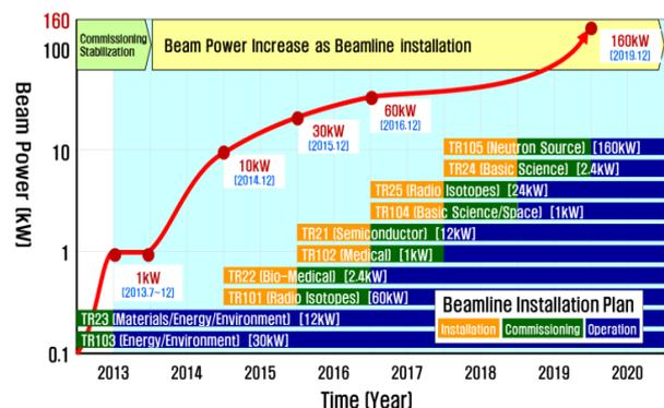
Fig. 11. Beam power and beam lines upgrade plan.
