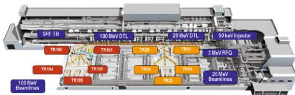
Fig. 1. Layout of the KOMAC accelerator building
