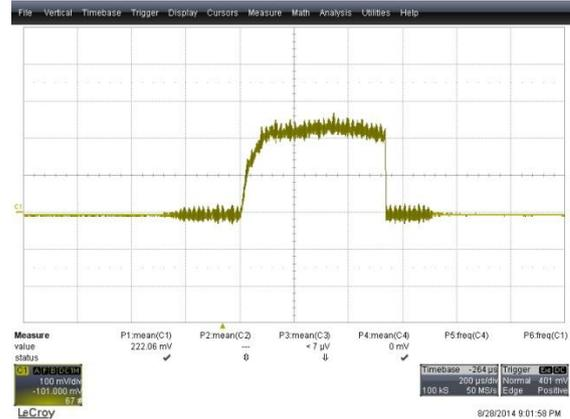
Fig. 4. Beam current signal (550 us)
