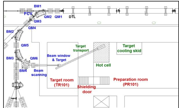
Fig. 9. Layout of RI production beam line and target room.
