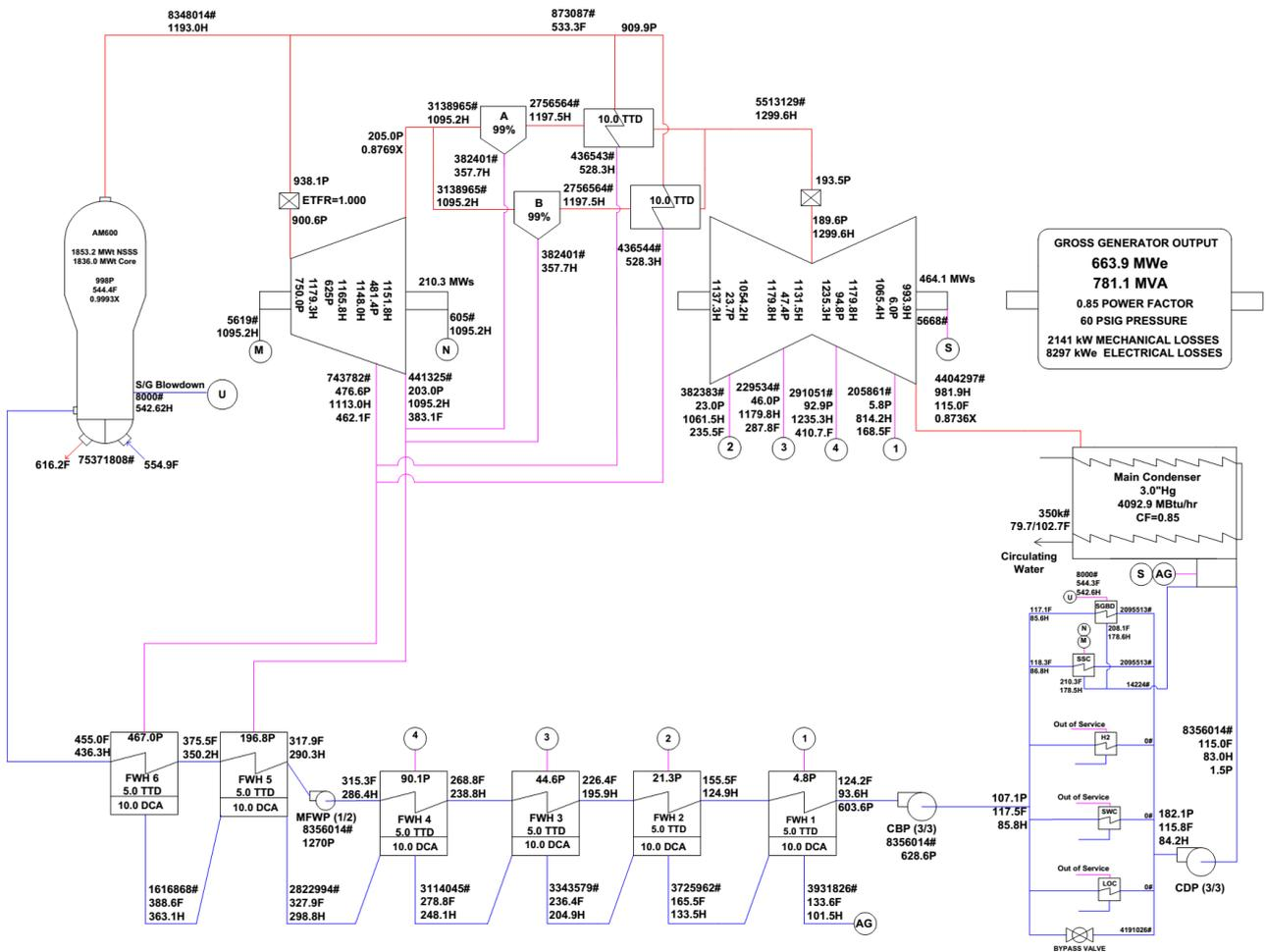
Fig.5. AM600 Heat balance diagram showing component count and arrangement.
