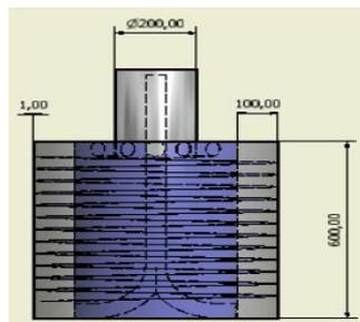
Fig. 1. The conceptual drawing of the water-filled beam dump
