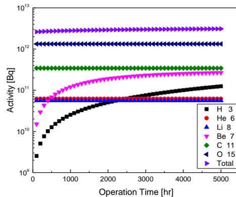
Fig.3. Activities of radionuclides produced in water during the operation.
