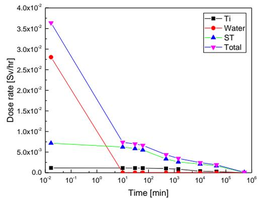
Fig.9. Dose rates from each component as a function of cooling time.
