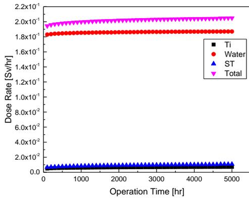
Fig.5. Dose rates from each component during the operation
