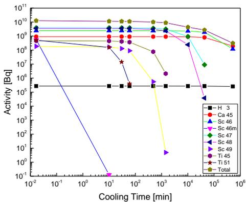
Fig.6. Activities of radionuclides produced in titanium as a function of cooling time.
