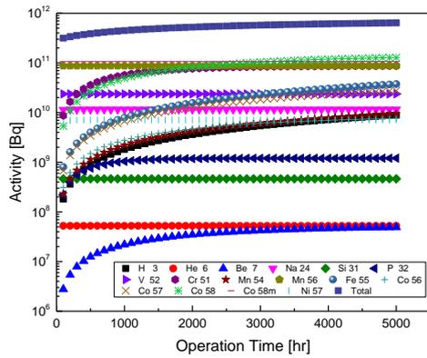
Fig.4. Activities of radionuclides produced in ST304 during the operation.
