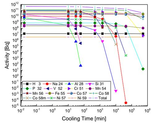
Fig.7. Activities of radionuclides produced in water as a function of cooling time.
