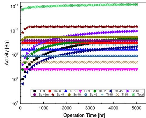
Fig.2. Activities of radionuclides produced in titanium during the operation.
