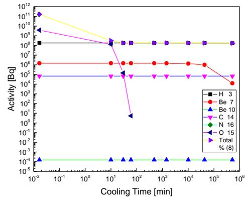
Fig.8. Activities of radionuclides produced in ST304 as a function of cooling time.
