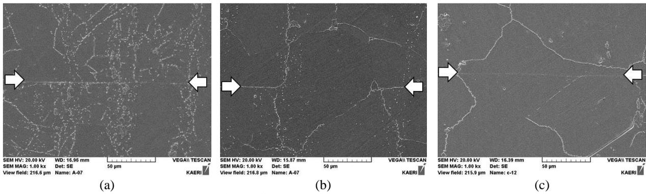
Fig. 2. Cross-sectional SEM micrographs of the diffusion-bonded Hastelloy-X: (a) HX-A, (b) HX-B, and (c) HX-C
