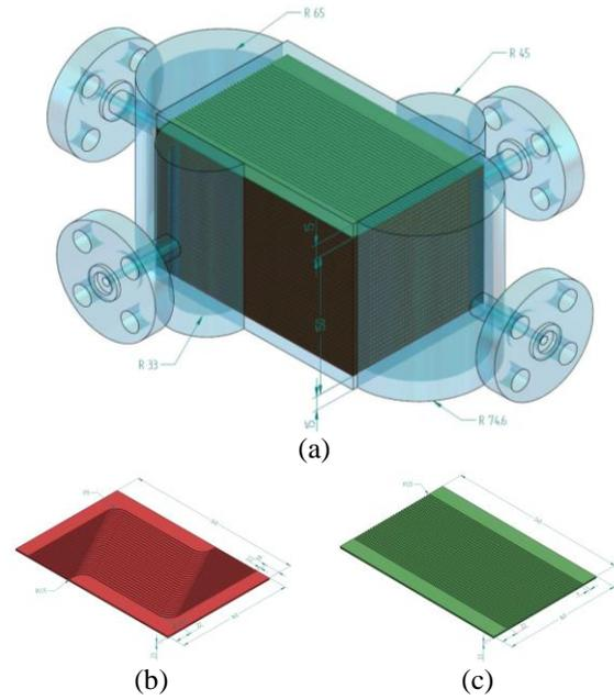
Fig. 1. An advanced small-scale microchannel-type PHE: (a) overall view, (b) plates with microchannel (primary side), and (c) plates with microchannel (secondary side)
