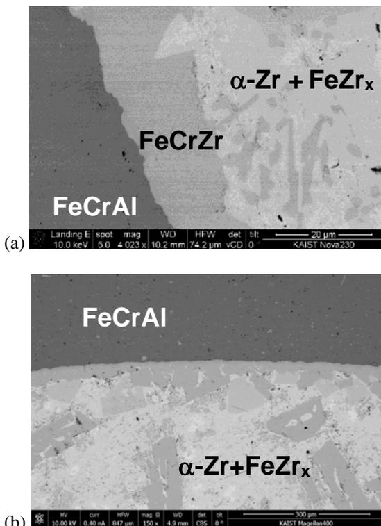
Fig. 3. SEM cross section microstructures of double wall cladding tubes annealed at (a) 1200°C for 1 hour and (b) 1300°C for 1 hour.
