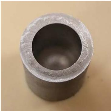
Fig. 2. The melting of Zircaloy-4 inner layer of a double wall cladding tube after annealing at 1150°C.
