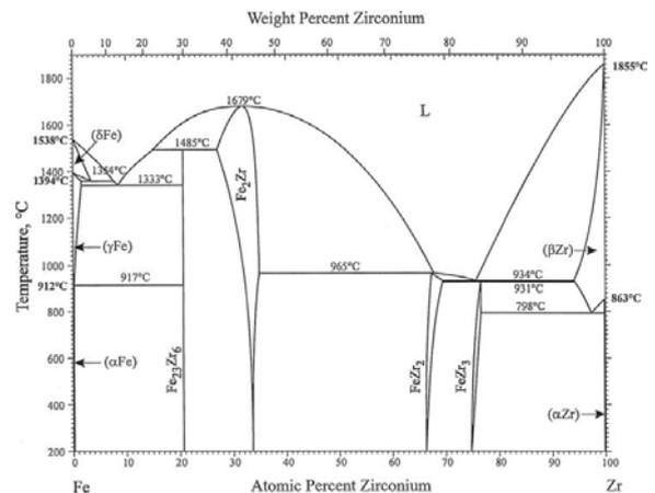
Fig. 1. The Fe-Zr binary phase diagram [12]
