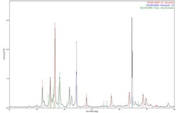
Fig. 4. X-ray diffraction pattern of a double wall cladding tube annealed at 1150°C for 1 hour.
