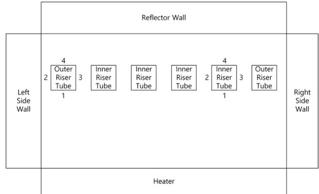
Fig. 3 Cross Sectional View of Risers & Cavity
