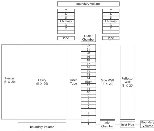
Fig. 2 GAMMA+ Nodalization
