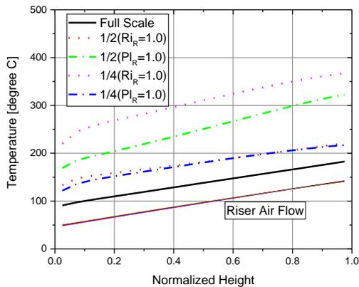
(b) Riser Wall Temperature & Air Flow Temperature
