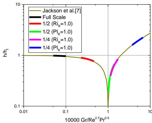
Fig. 5 Theoretical prediction of General Features of Mixed Convection Heat Transfer in Vertical Tubes with the GAMMA+ Analysis Conditions
