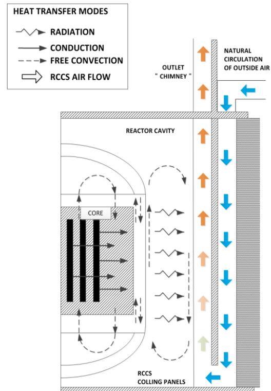
Fig. 1 Heat Removal Mechanism in RCCS
