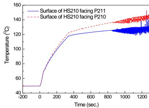
Fig. 10. Fuel surface temperatures at the fuel plate (FCB)
