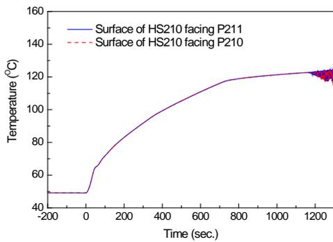
Fig. 6. Fuel surface temperatures at the fuel plate (NNC)
