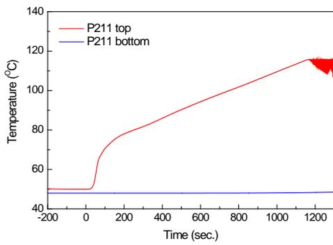
Fig. 4. Coolant temperatures at the flow channel (NNC)
