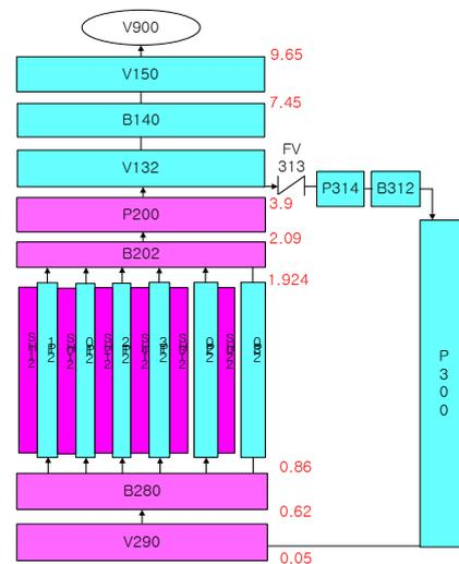
Fig. 1. Node diagram for RELAP5 simulation
