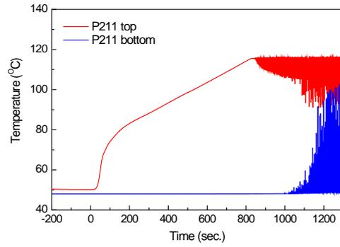
Fig. 8. Coolant temperatures at the flow channel (FCB)
