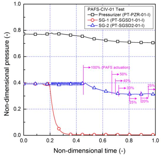
Fig. 4. Primary and secondary system pressure.
