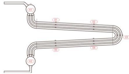
Fig. 2. Design of the PCHX (dimension in mm).
