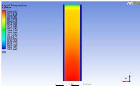
Fig.3 liquid temperature distribution
