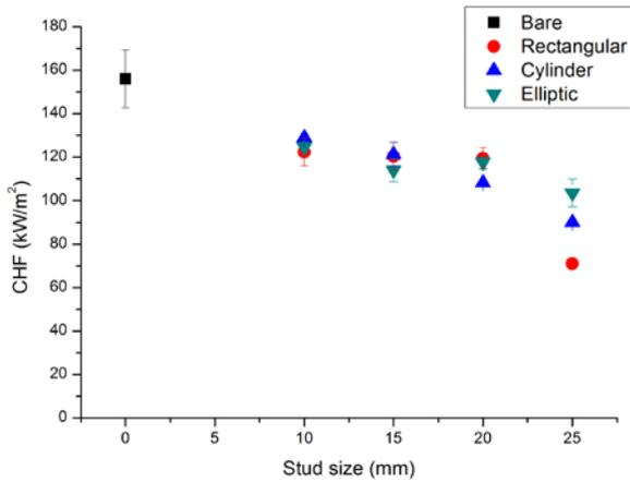
Fig. 5. CHF value with respect to the stud shape and size.
