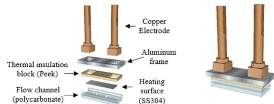
Fig. 2. Schematic diagram of the test section
