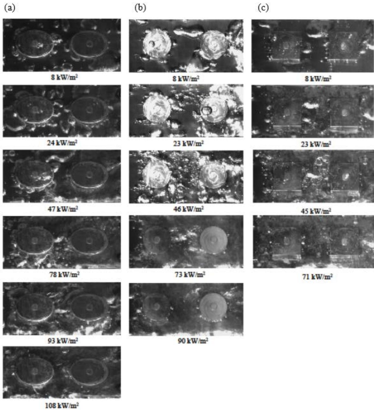
Fig 7. Visualization on the studs' shape with stud size of 25 mm; (a) elliptic, (b) cylinder, and (c) rectangular
