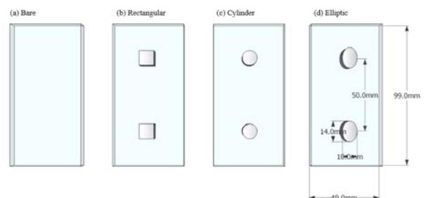
Fig. 3. Schematic diagram of Stud shapes
