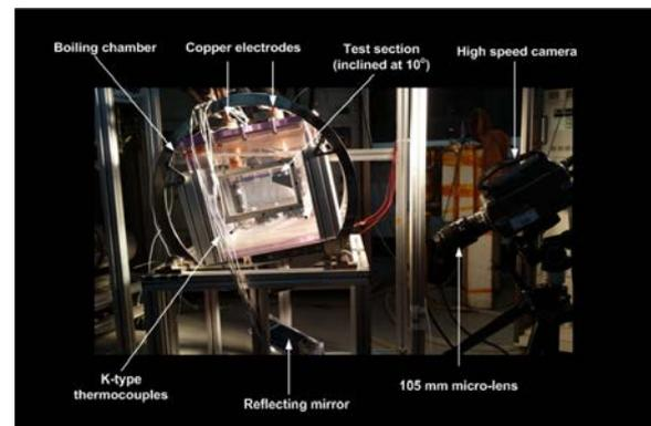
Fig 1. Photo of pool boiling apparatus
