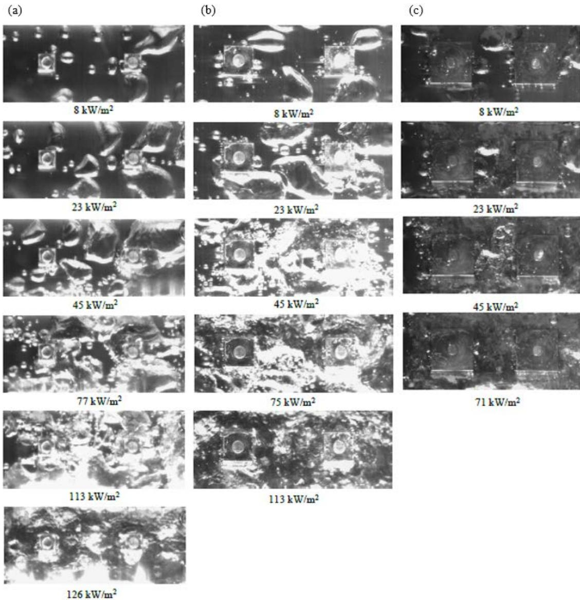
Fig 6. Visualization on the rectangular stud; (a) 10 mm, (b) 15 mm, and (c) 25 mm
