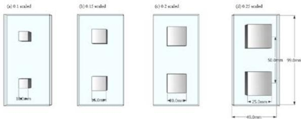
Fig. 4. Schematic diagram of Stud sizes
