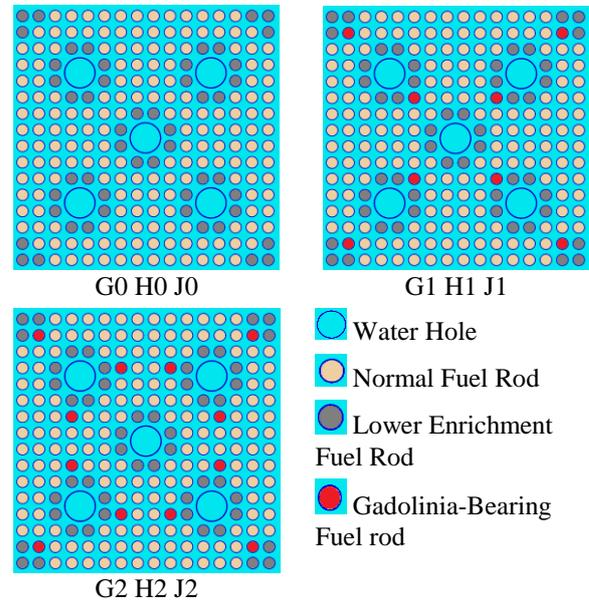
Fig. 1. Configuration of the fuel assemblies in HBN#3 Cycle6.
