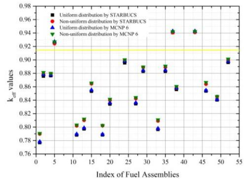
Fig. 7.  $k_{eff}$  values for the cask with various fuel assemblies for the cooling time of 30 years.
