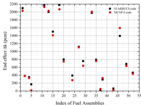
Fig. 10. End effects (pcm) of various fuel assemblies for the cooling time of 30 years.
