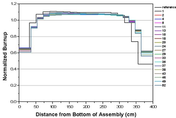
Fig. 4. Normalized axial burnup distributions for the reference [1] and 20 NFAs of Cycle 6.
