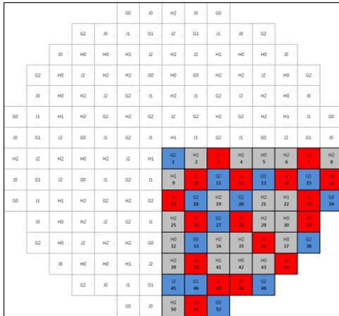
Fig. 3. Loading pattern in the reactor core of Cycle 6.
