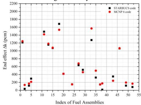
Fig. 9. End effects (pcm) of various fuel assemblies for the cooling time of 20 years.
