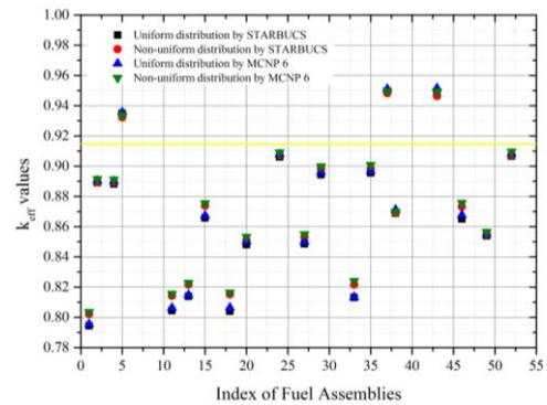
Fig. 6.  $k_{eff}$  values for the cask with various fuel assemblies for the cooling time of 20 years.
