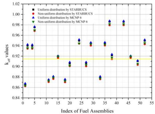
Fig. 5.  $k_{eff}$  values for the cask with various fuel assemblies for the cooling time of 0 year.
