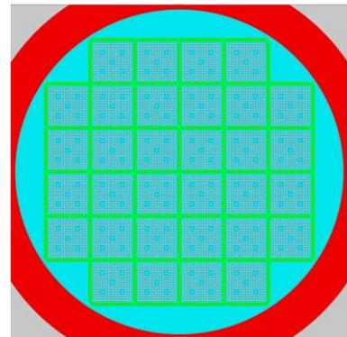
Fig. 2. Radial cross section of the GBC-32 dry storage cask.
