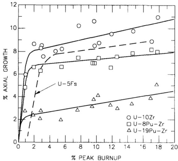
Fig. 5. Fuel Length Increases in Various Metallic Fuels as a Function of Burnup [5]
