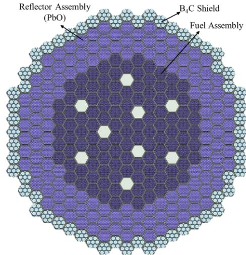
Fig 3. Modified PGSFR core axial layout
