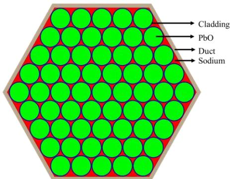
Fig 2. PbO reflector assembly geometry
