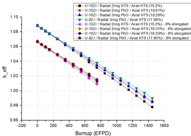
Fig 6. Single batch depletion calculation results
