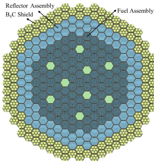
Fig. 1. PGSFR core radial layout [1].
