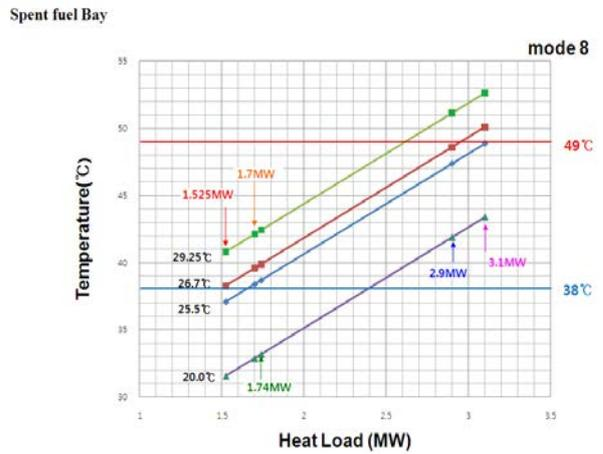
Fig. 6. Bulk temperature in spent fuel bay for operating modes 8 and 9
