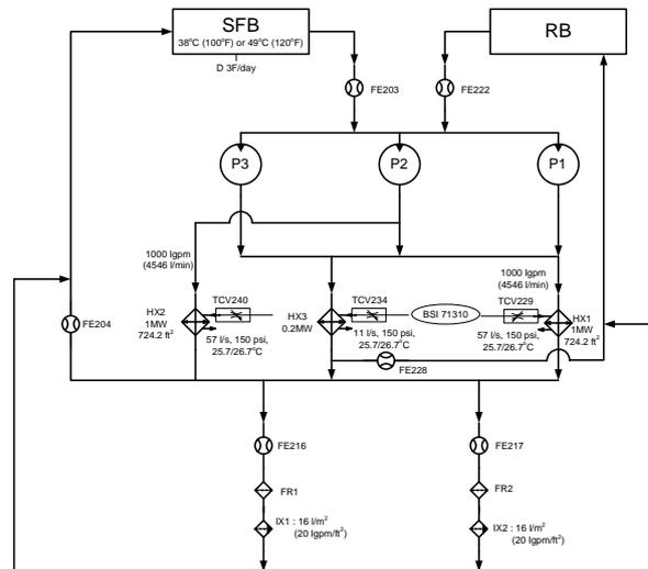
Fig. 1. Schematic diagram of the CANDU spent fuel bay cooling system
