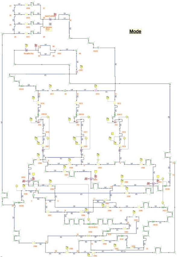
Fig. 3. Flowmaster modeling for spent fuel bay cooling and purification system
