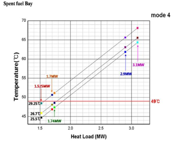
Fig. 5. Bulk temperature in spent fuel bay for operating modes 3, 4, 5, 6 and 7
