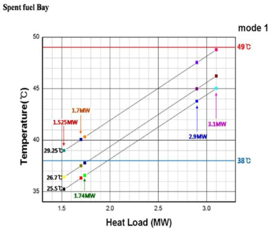
Fig. 4. Bulk temperature in spent fuel bay for operating modes 1, 2 and 10
