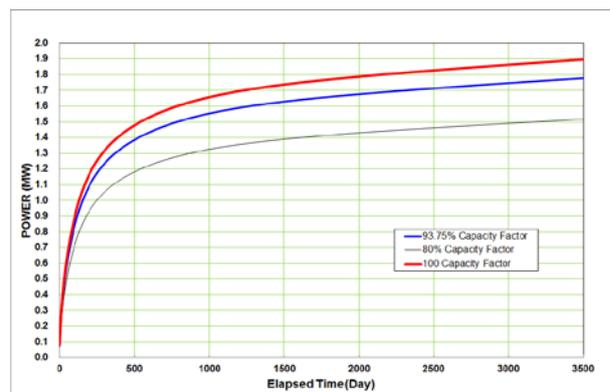
Fig. 2. Heat loads with various capacity factor refueling rates
