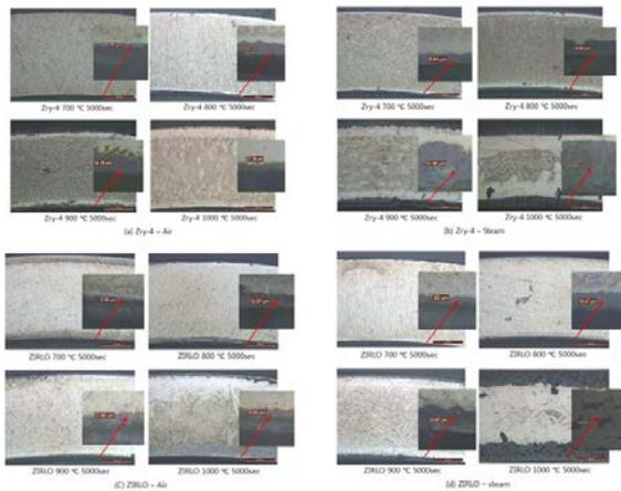
Figure 7. OM image of microstructure of no-CRUD layer in Zr alloy interior by each temperature
