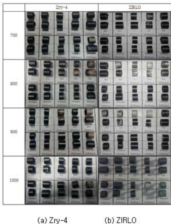
Figure 4. Image of 700~1000 °C oxidation specimen exterior in steam and air atmosphere.
