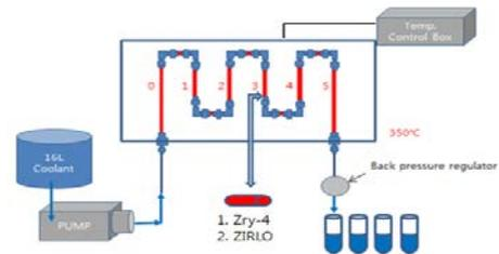
Figure 1. Mimetic diagram of CRUD-forming experimental device.
