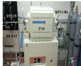
Figure 2. High-temperature discontinuous measurement oxidation device (tube furnace).
