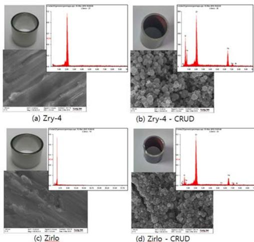
Figure 3. SEM image of no-CRUD and CRUD in Zr alloy interior.
