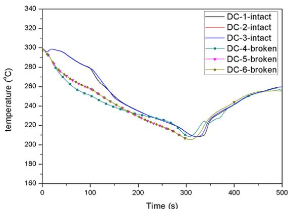
Figure 9. Asymmetric Temperatures of Downcomer Nodes
