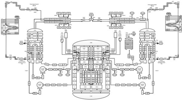
Figure 1. MARS-KS APR+ Nodalization.
