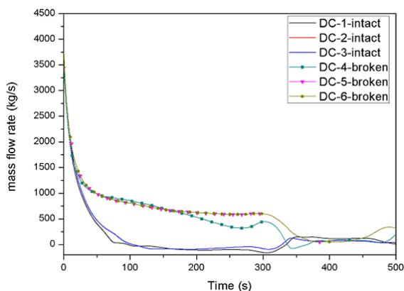
Figure 8. Asymmetric Natural Circulation Flows Of Downcomer Nodes
