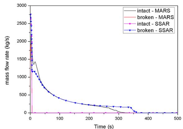
Figure 2. Steam flows of Intact and Broken SGs
