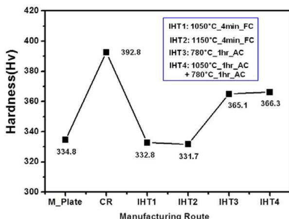
Fig. 1. Effects of the cold rolling and intermediate heat treatments on the Vickers microhardness of 10Cr FM ODS steel.
