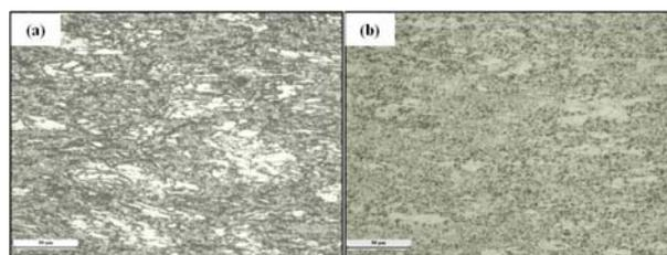
Fig. 2. Optical micrographs of (a) hot-extruded and (b) cold-rolled 10Cr-1Mo FM ODS steels.
