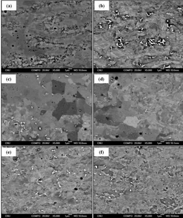
Fig. 3. SEM micrographs of the grain morphology for 10Cr FM ODS steels in different intermediate heat treatment conditions are presented: (a) hot-extruded, (b) cold rolled, (c) IHT1, (d) IHT2, (e) IHT3, and (f) IHT4
