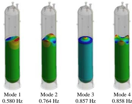
Fig. 1. Sloshing modes of coolant inside the PZR
