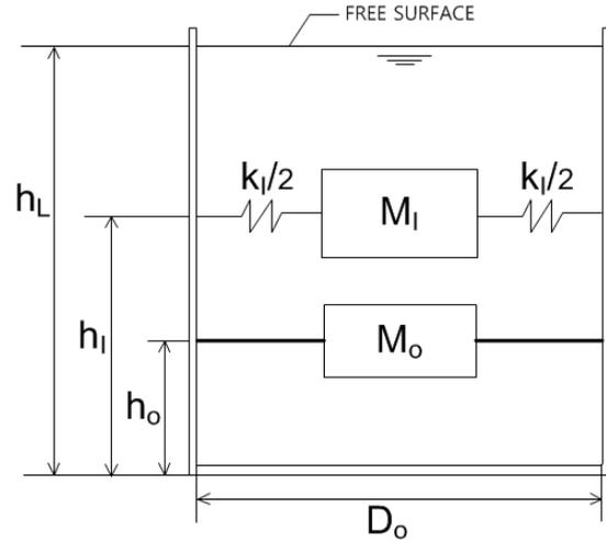
Fig. 2. Equivalent dynamic system of a cylindrical tank
