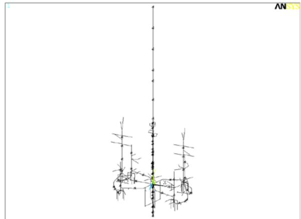
Fig. 3. RCS seismic analysis model
