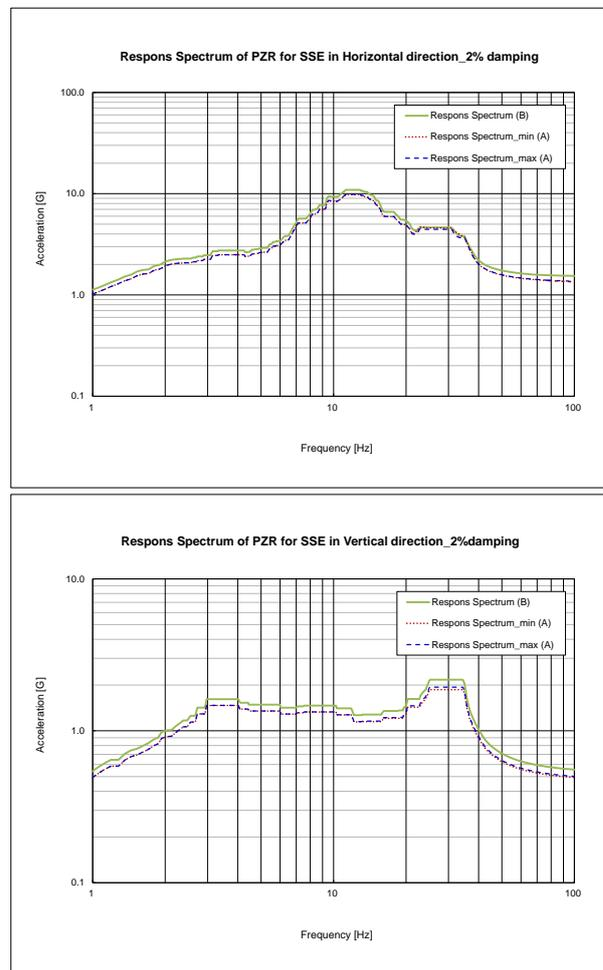
Fig. 4. Comparison of response spectra of conventional design with that of seismic analysis considering effect of PZR sloshing
