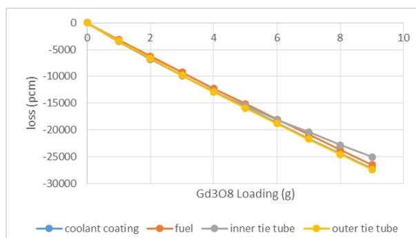
Fig. 7. Reactivity loss due to Gadolinium when inserted into different locations in the Inverse Alpha (2:1) core with loadings from 0 g to 9 g of Gadolinia.
