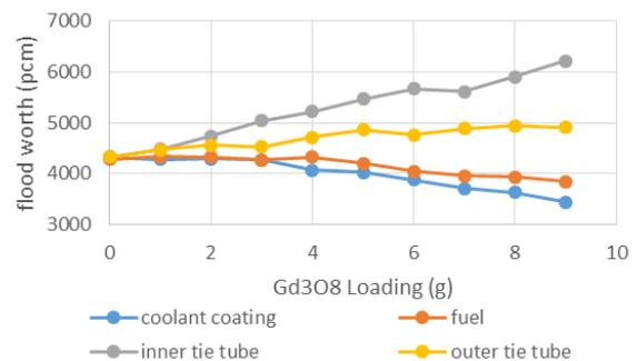
Fig. 8. Flood worth for different poison locations as a function of Gadolinia loading in the core.
