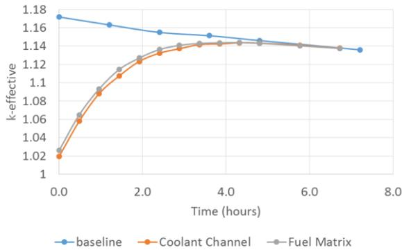
Fig. 9. Depletion of the core at 450 MW for 8 hours with the poison implemented in the fuel matrix and the coolant channel.
