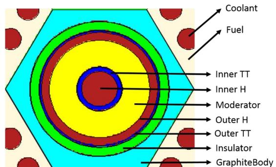
Fig. 2. Moderator and fuel element geometries.
