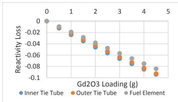
Fig. 4. Reactivity loss due to Gadolinium when inserted into different locations in the Bulls-Eye (1:1) core.
