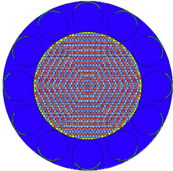
Fig. 3. Reference core radial geometry using the Bulls-Eye configuration (1:1).
