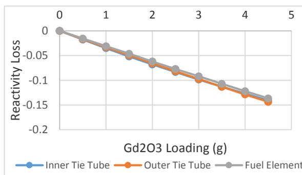
Fig. 5. Reactivity loss due to Gadolinium when inserted into different locations in the Inverse Alpha (2:1) core.
