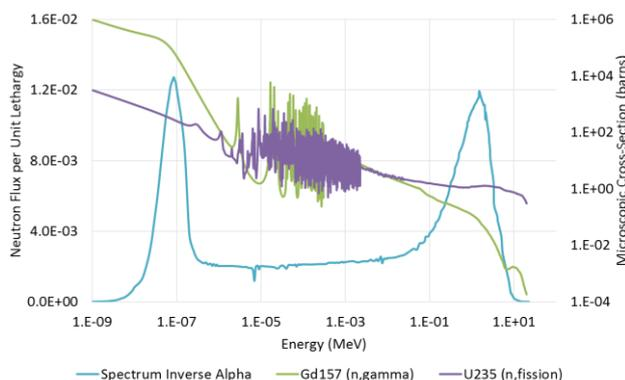
Fig. 6. Absorption cross-section of  $^{157}\text{Gd}$  along with the fission cross-section of  $^{235}\text{U}$  and the core average absorption neutron flux of the Inverse-Alpha (2:1) reference core.
