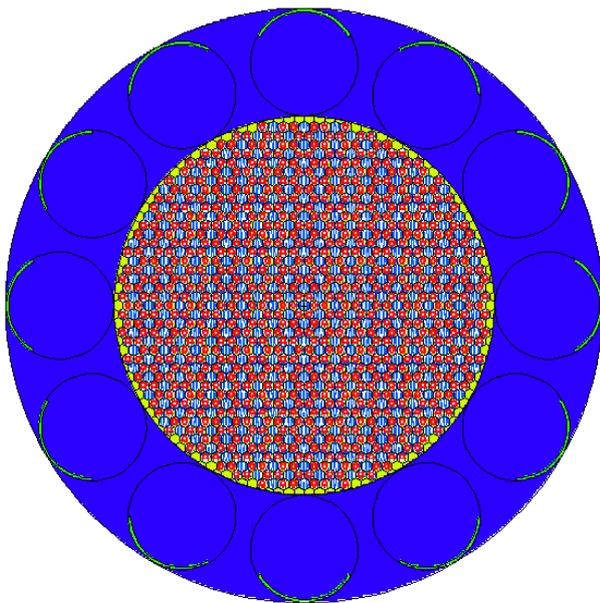
Fig. 2. Reference core radial geometry using the Inverse Alpha configuration (2:1).
