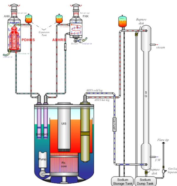
Figure 2 Schematic of the PGSFR
