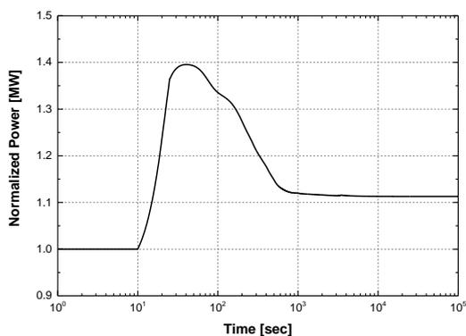
Figure 3 Reactor power during the UTOP event for nominal fuel conditions
