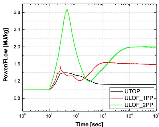
Figure 7 Power/Flow during the DEC events
