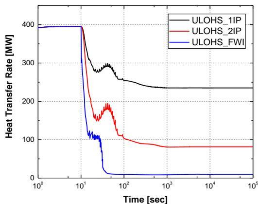
Figure 5 Heat transfer rate in the steam generators for nominal fuel conditions during the ULOHS events
