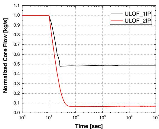
Figure 4 Normalized core flows of nominal fuel conditions for the ULOF events
