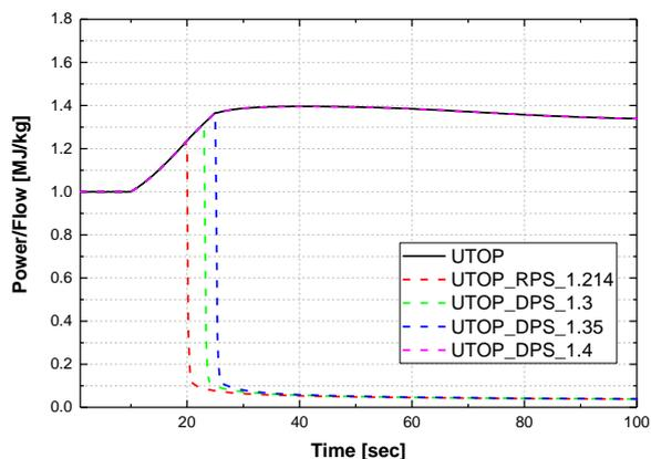
Figure 8 Power/Flow during the UTOP event for different set-points of DPS
