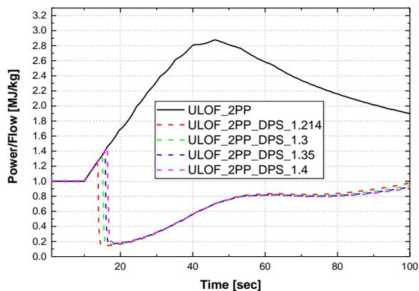
Figure 10 Power/Flow during the ULOF\_2PP event for different set-points of DPS
