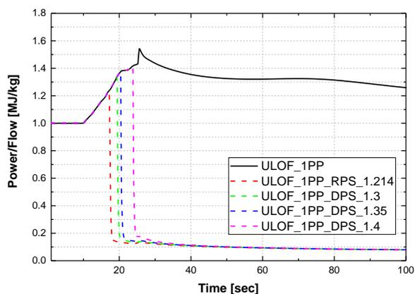
Figure 9 Power/Flow during the ULOF\_1PP event for different set-points of DPS
