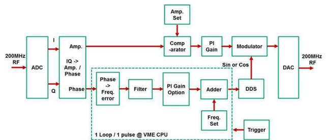
Fig. 2. The FPGA control logic layout
