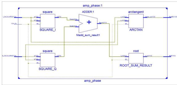
Fig. 4. Implement of the module-2 in the FPGA
