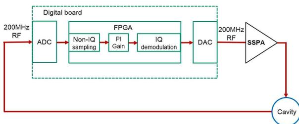
Fig. 1. Helium RFQ RF system layout
