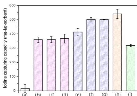
Fig. 2. Iodine capturing capacities in static air for (a) SBA-15, (b) Bi-SBA-15-SH1, (c) Bi-SBA-15-SH2, (d) Bi-SBA-15-SH3, (e) Bir-SBA-15-SH1, (f) Bir-SBA-15-SH2, (g) Bir-SBA-15-SH3, (h) Bir-SBA-15-SH2A, and (i) AgX (tested at 150 °C).
