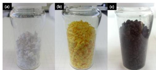
Fig. 1. Pictures of (a) thiol-functionalized SBA-15, (b) bismuth-embedded SBA-15 (before heat-treatment), and (c) bismuth-embedded SBA-15 (after heat-treatment).
