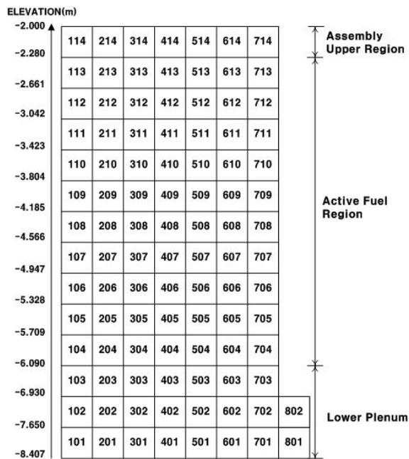
Fig. 2. The core nodalization of OPR1000 for MELCOR
