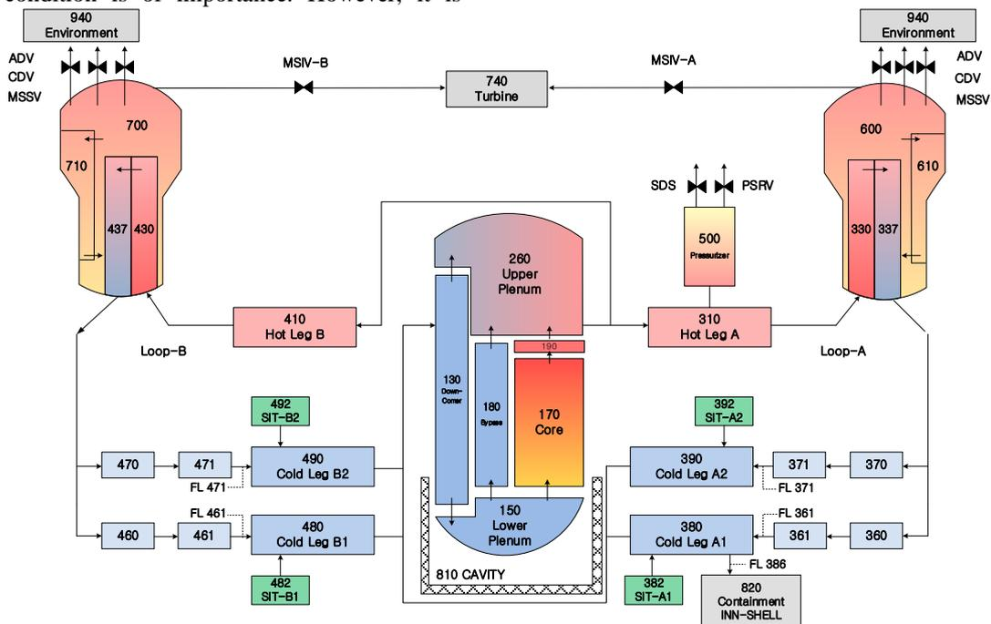
Fig. 1. Nodalization of MELCOR input model for OPR1000
