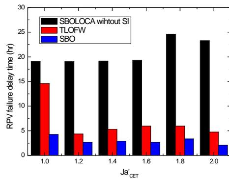
Fig. 4. RPV Failure Delay Time of Case with mitigation
