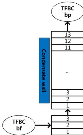
Fig. 6. The nodalization schematic of KAIST tests
