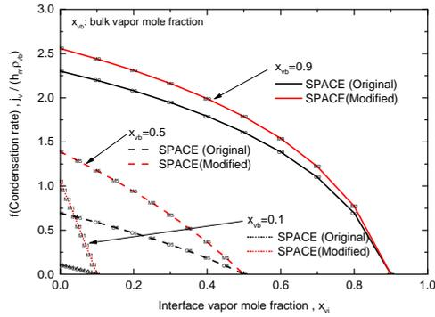
Fig. 1. Comparison of tendency of condensation rate for the cases of 0.1, 0.5, and 0.9 of bulk vapor mole fractions ( $x_{vb}$ ) according to the change of vapor mole fraction at liquid/gas interface ( $x_{vi}$ )
