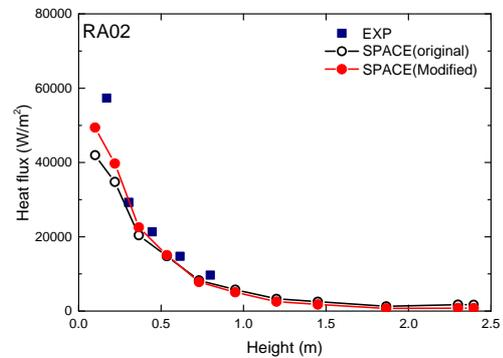
Fig. 8 Comparison of heat flux using SPACE with KAIST reflux condensation data for test RA02
