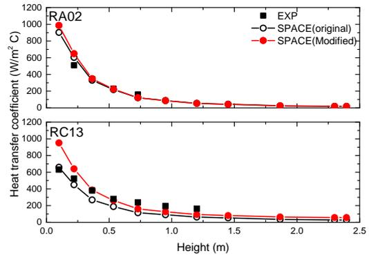
Fig. 7. Comparison of HTC using SPACE for test RA02 & RC13
