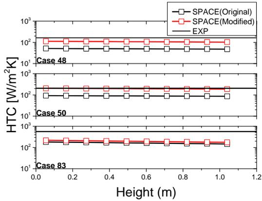
Fig. 5. Comparison of HTC with averaged HTC for UW condensation data
