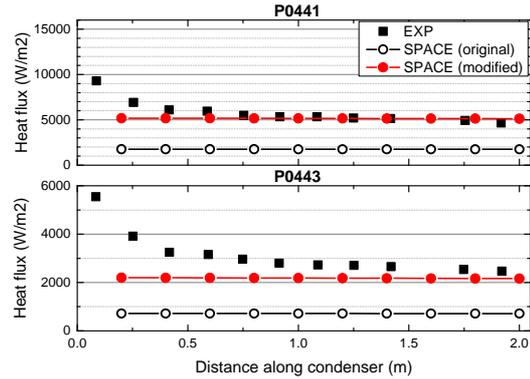
Fig. 3. Comparison of heat flux using SPACE with COPAIN data for tests P0441 and P0443
