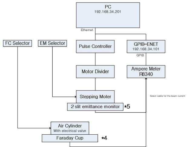
Fig. 9. Schematic diagram of the beam monitor control
