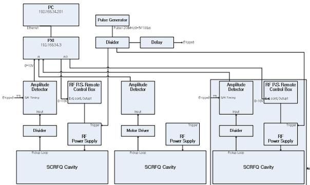
Fig. 5. Schematic diagram of the RF voltage control
