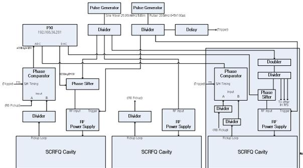
Fig. 6. Schematic diagram of the phase lag between cavities
