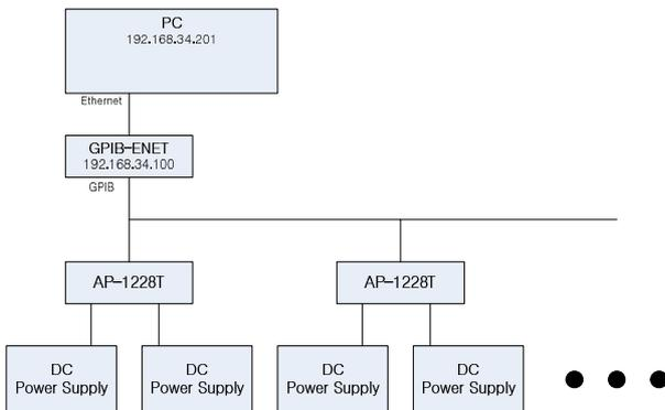
Fig.7. Schematic diagram of the Magnet Power Supply
