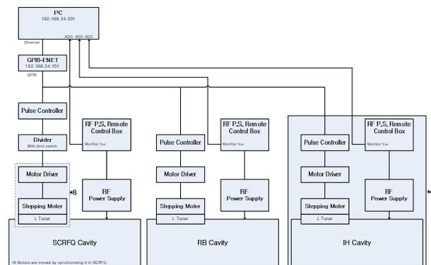
Fig. 4. Schematic diagram of the cavity resonance frequency control
