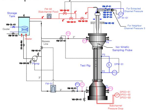
Fig. 2. Schematic of the Test Facility.
