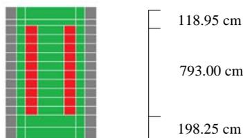
Fig. 2. Axial layer meshes.
