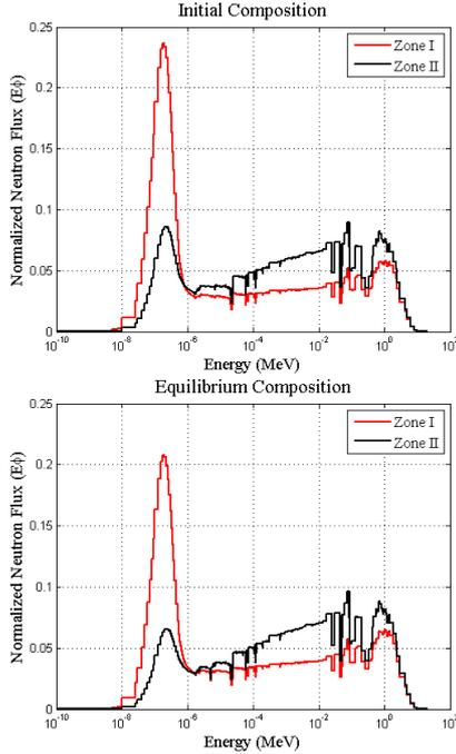
Fig. 5. Normalized neutron spectrum of two-cell method for initial and equilibrium core
