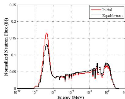
Fig. 3. Normalized neutron spectrum of single-cell method for initial and equilibrium core
