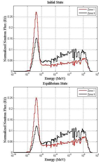
Fig. 7. Normalized neutron spectrum of whole core model for initial and equilibrium core
