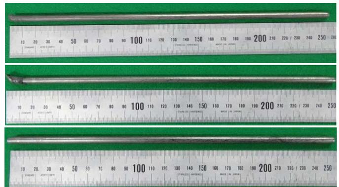
Fig. 1. (a) U-10wt%Zr-3wt.%RE, (b) U-10wt%Zr-7wt.%RE, and (c) U-10wt%Zr-10wt.%RE fuel slug ( $\Phi 5 \times L 250$  mm), fabricated by modified injection casting.
