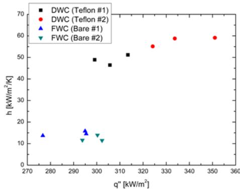
Fig. 4. Condensation on vertical plate experimental result
