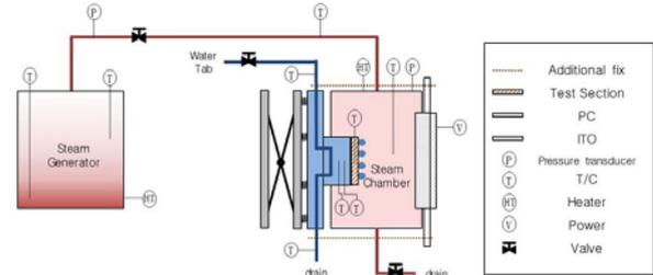
Fig. 3. Condensation on vertical plate experimental loop
