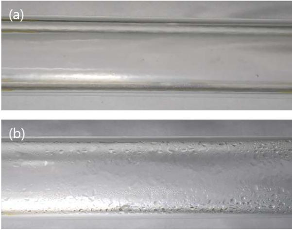
Fig. 2. Visualization inside horizontal borosilicate pipes. (a) FWC was showed inside a bare borosilicate pipe, (b) DWC was showed inside a Teflon coated pipe. Images were taken in top view.
