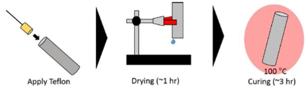
Fig. 1. Inside-a-pipe Teflon coating method
