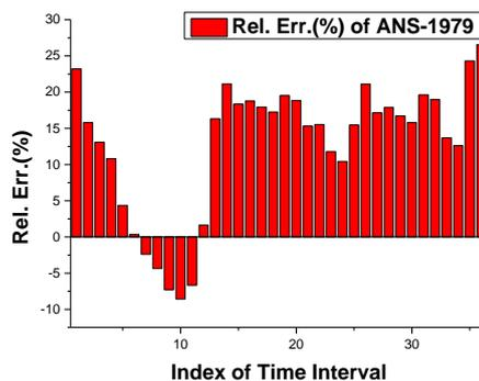
Fig. 14. Relative Differences of Whole Core Decay Heat Power for Each Time Interval
