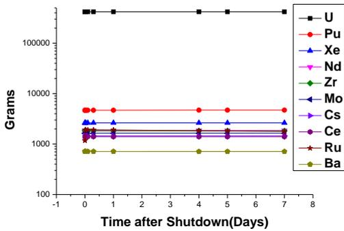
Fig. 4. The Change of the Mass of the Top 10 Elements
