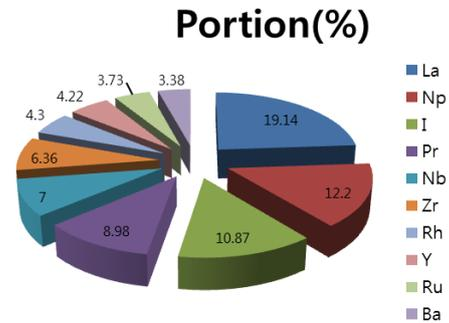
Fig. 11. Initial Decay Heat of the Top 10 Elements
