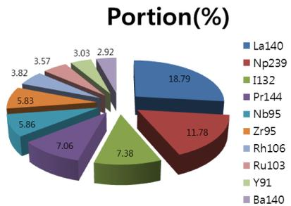
Fig. 9. Initial Decay Heat of the Top 10 Nuclides
