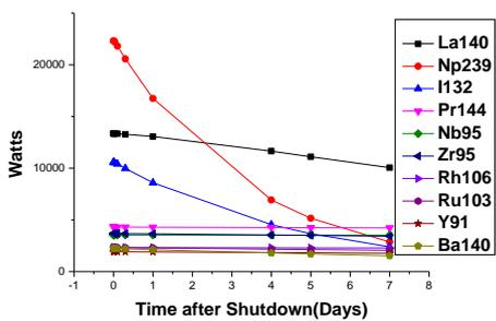
Fig. 10. The Change of the Decay Heat of the Top 10 Nuclides
