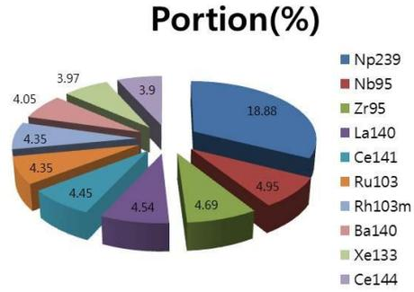
Fig. 5. Initial Radioactivity Ratio of the Top 10 Nuclides
