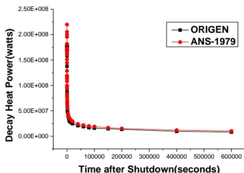
Fig. 13. Comparison of Whole Core Decay Heat Power with Time After Shutdown
