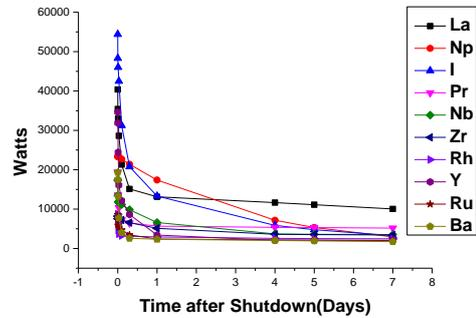
Fig. 12. The Change of the Decay Heat of the Top 10 Elements
