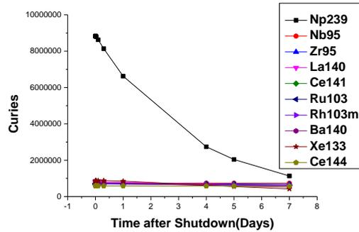
Fig. 6. The Change of the Radioactivity of the Top 10 Nuclides
