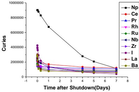
Fig. 8. The Change of the Radioactivity of the Top 10 Elements
