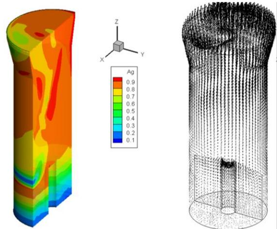
Fig. 3 void fraction distribution and velocity vectors
