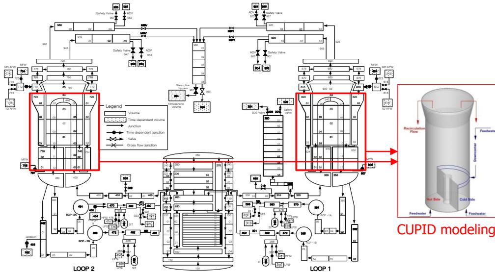
Fig. 2 APRI400 nodalization for CUPID/MARS coupled simulation
