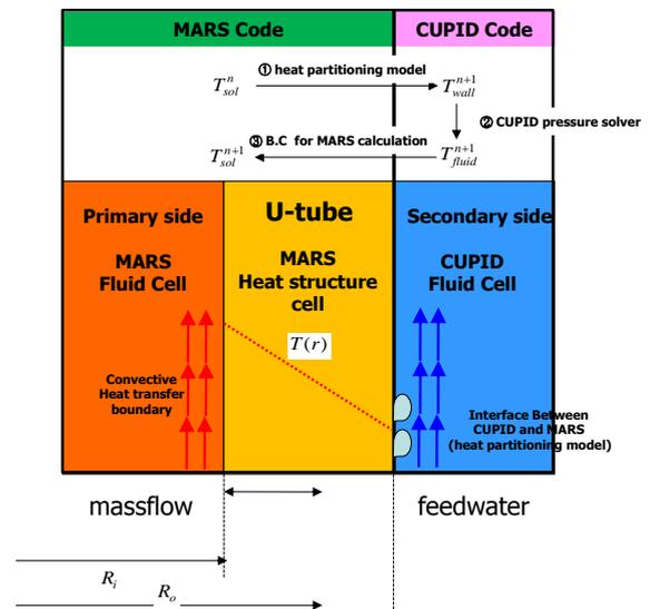
Fig. 1 Coupling method between CUPID and MARS.
