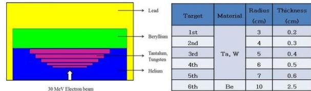
Fig. 1. Structure and material of the target.
