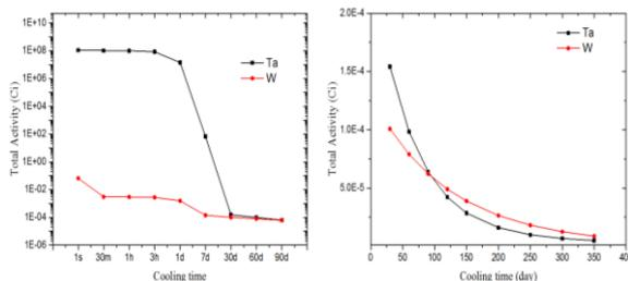
Fig. 4. Total activity of target for cooling of 90 and 350 days.
