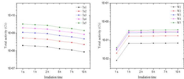
Fig. 2. Total activity of Ta and W targets for irradiation time.
