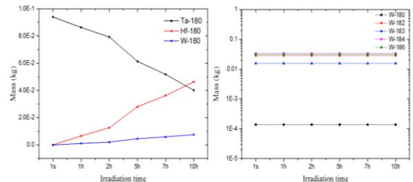
Fig. 3. Mass of Ta and W targets for irradiation time.
