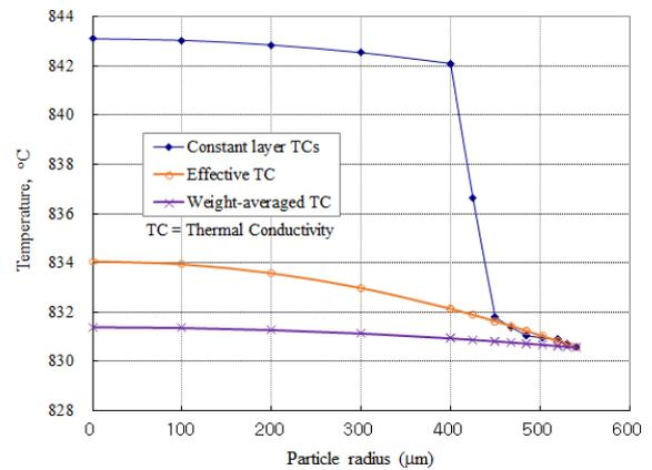
Fig. 4. Temperature Distribution within a TRISO.
