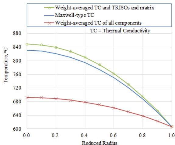
Fig. 6. Temperature Distribution within an FCM Fuel Pellet.
