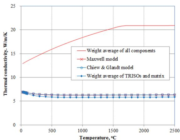
Fig. 5. Effective Thermal Conductivities of an FCM Fuel Pellet.
