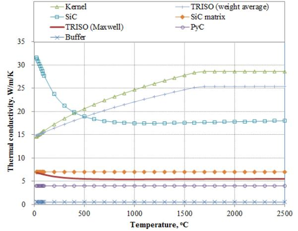
Fig. 3. Thermal Conductivities of TRISO Materials and SiC Matrix
