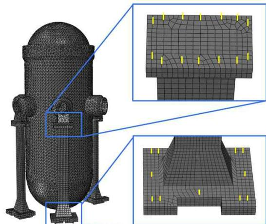
Fig. 1 Combined FE mode and location of anchor bolts
