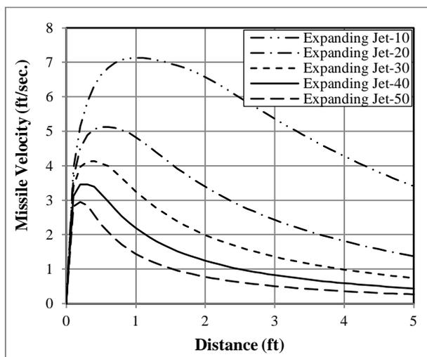
Fig. 5. Missile Velocities for Pressure Approach model
