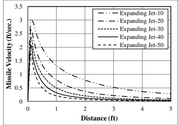
Fig. 3. Missile Velocities for Direct Approximation Model
