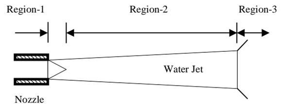
Fig. 1. Anatomy of High Speed Water Jet in Air
