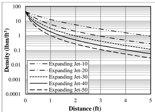
Fig. 4. Density change for Pressure Approach Model
