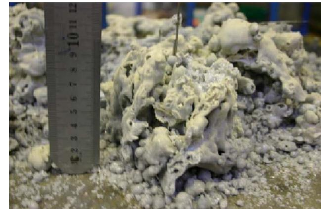
Fig 4. Debris beds formed in DEFOR-E test [2]
