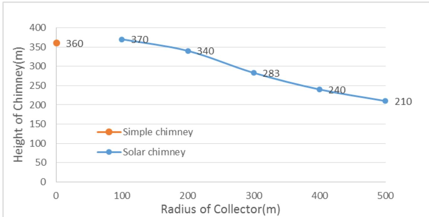
Height of simple and solar chimney for removing  $200\text{MW}_{\text{th}}$  heat
