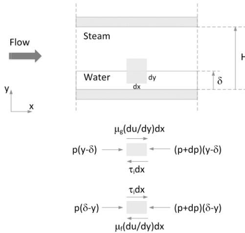
Fig. 1. Physical model for steam condensation in horizontal plate
