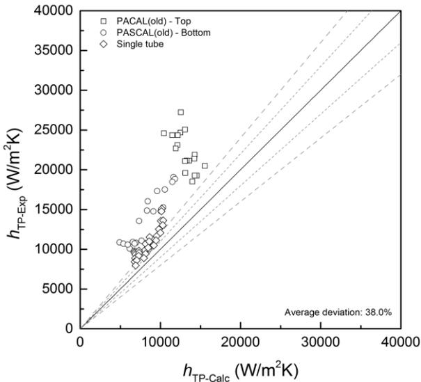
Fig. 2. Comparison for the total condensation heat transfer coefficient using Shah (2009) correlation
