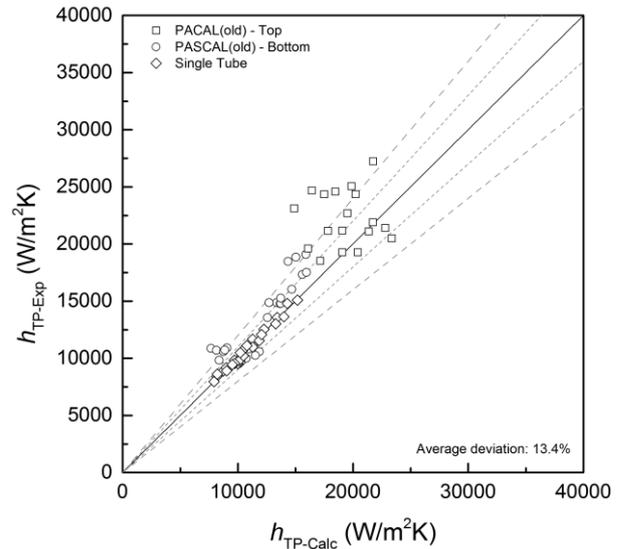
Fig. 3. Comparison for the total condensation heat transfer coefficient using the derived slip ratio model
