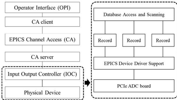
Fig. 3: Software layer of the beam monitoring system using EPICS [2].
