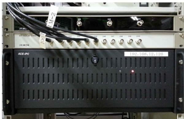
Fig. 2. Data acquisition system for beam monitors installed to klystron galley room.
