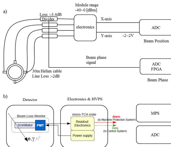
Fig. 1. Block diagram for data acquisition of beam signals from detectors for a) beam position monitor and b) beam loss monitor.
