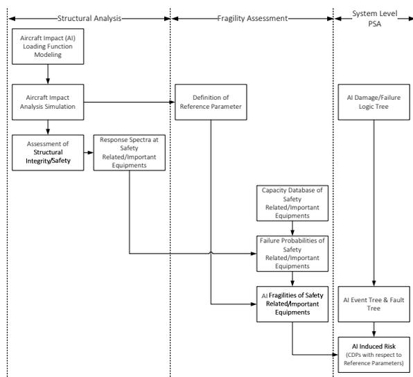
Fig. 1. Schematic diagram for the assessment procedure of the aircraft impact event induced risk of NPPs.
