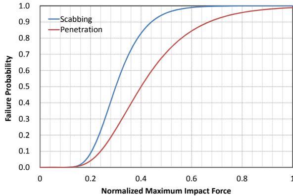
Fig.3 Example of the fragility curves for each failure mode.
