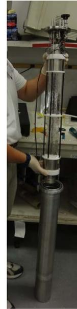
Fig. 17. Insertion of the entire detector assembly into the hermetically sealed detector enclosure. The enclosure was filled with dry argon to prevent moisture leaking into the enclosure.
