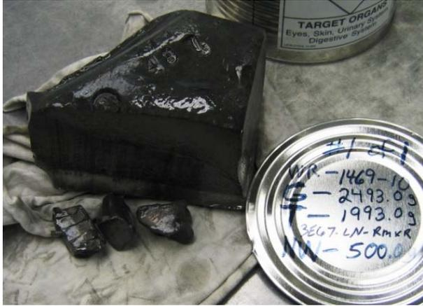
Fig. 3. A piece of unprocessed lithium-6 that has been soaked in mineral oil for long-term storage at Y-12 site.
