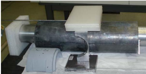
Fig. 20. Another neutron measurement setup to observe epithermal neutron response of the detector. Moderator was added behind the neutron source to observe the contribution of the backscattering neutrons.
