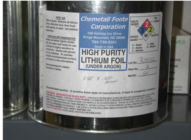
Fig. 5. The freshly processed rolls of lithium-6 foil were then pressure packed with dry argon gas for long-term storage. The cans were pressed sealed.
