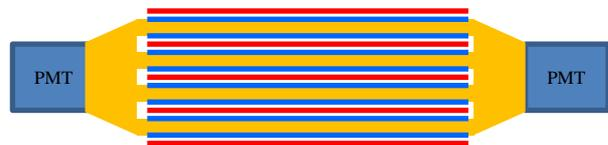
Fig. 1. Detector concept for the lithium sandwich detector. Li-6 metal neutron capturing foil, depicted in red, is sandwiched between scintillator films, in blue, laminated to the light guide strips. The dual side particle readout improves efficiency and pulse height distribution. The yellow body is the light guide material which transports photons to the PMTs and moderates fission neutrons.
