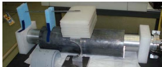
Fig. 18. Neutron response using a Cf-252 source. The measurement series started with no moderator material between the source and the detector that has been shielded with lead cylinder of 2 cm thickness.
