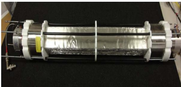
Fig. 16. The sandwich stack of light guide, plastic scintillator, and lithium foil is assembled, ready for insertion into the hermetically sealed container.
