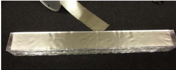
Fig. 15. The lithium foil pieces are cut and inserted between lightguides whose exterior surfaces are covered with plastic scintillator film.
