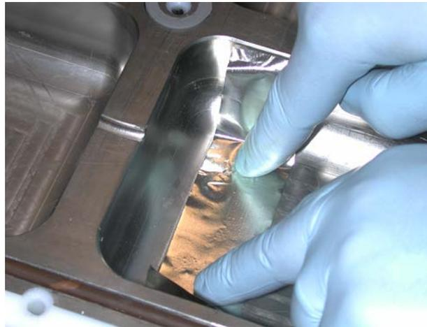
Fig. 6. A piece of lithium foil is cut with a pair of scissors and pressed on to a metalized surface of a lithium-6 neutron-capture pulse mode ion chamber.
